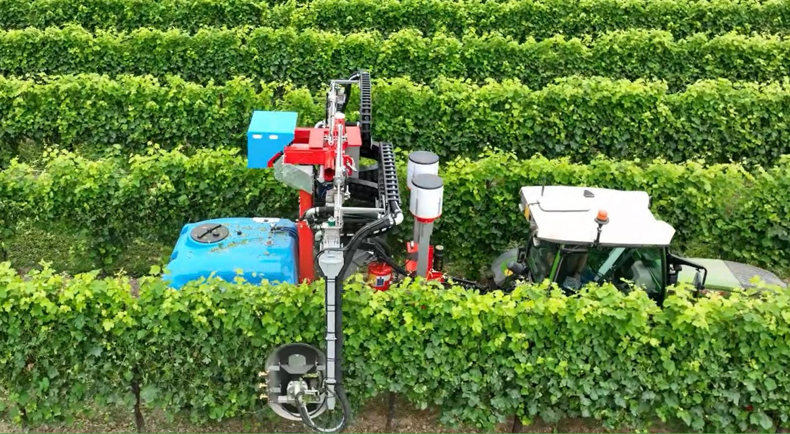
**Defoliation** - Machine in the field during the targeted treatment of two rows
